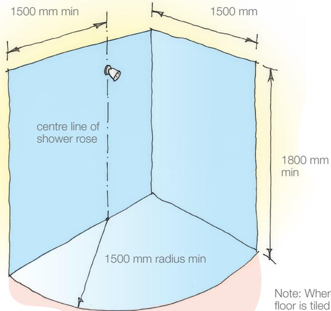
Note: Where the whole floor is tiled BRANZ recommends that the waterproof membrane is extended under the whole floor.
