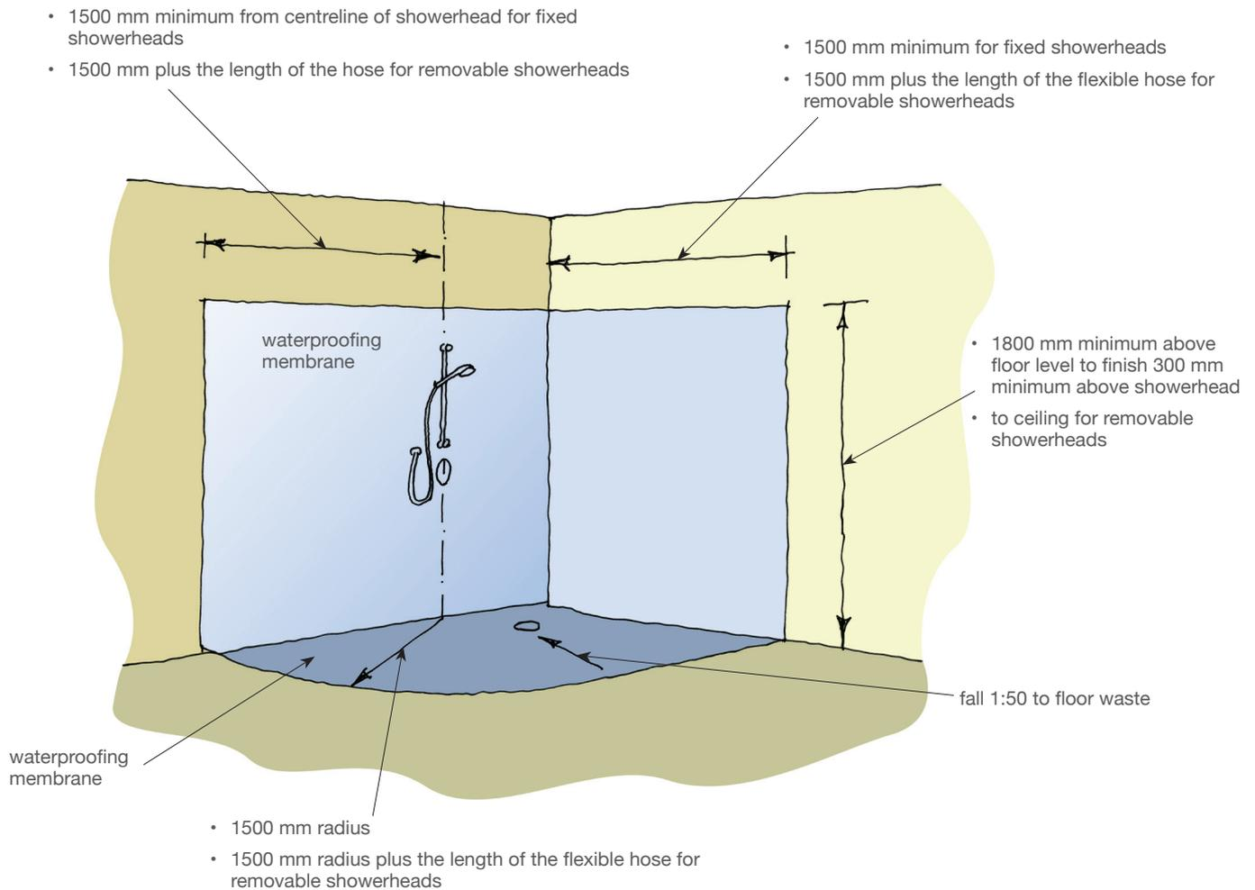
1. Waterproofing the entire floor when the floor is tiled is recommended.
