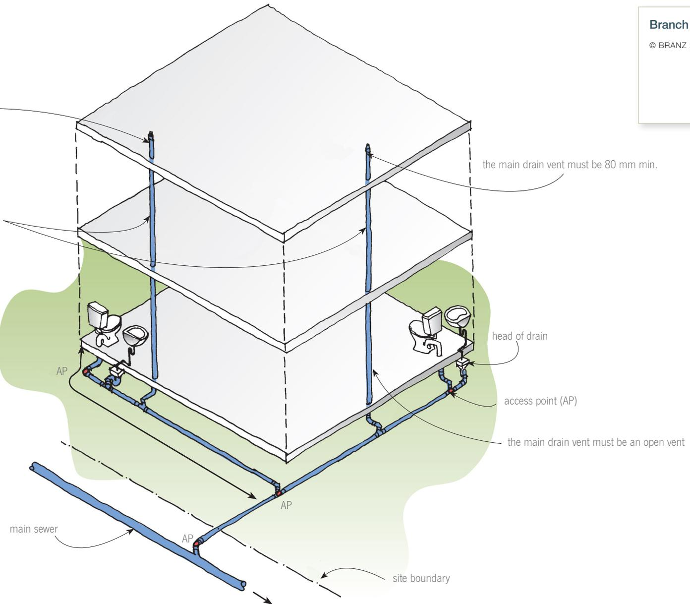
the main drain vent must be 80 mm min.
