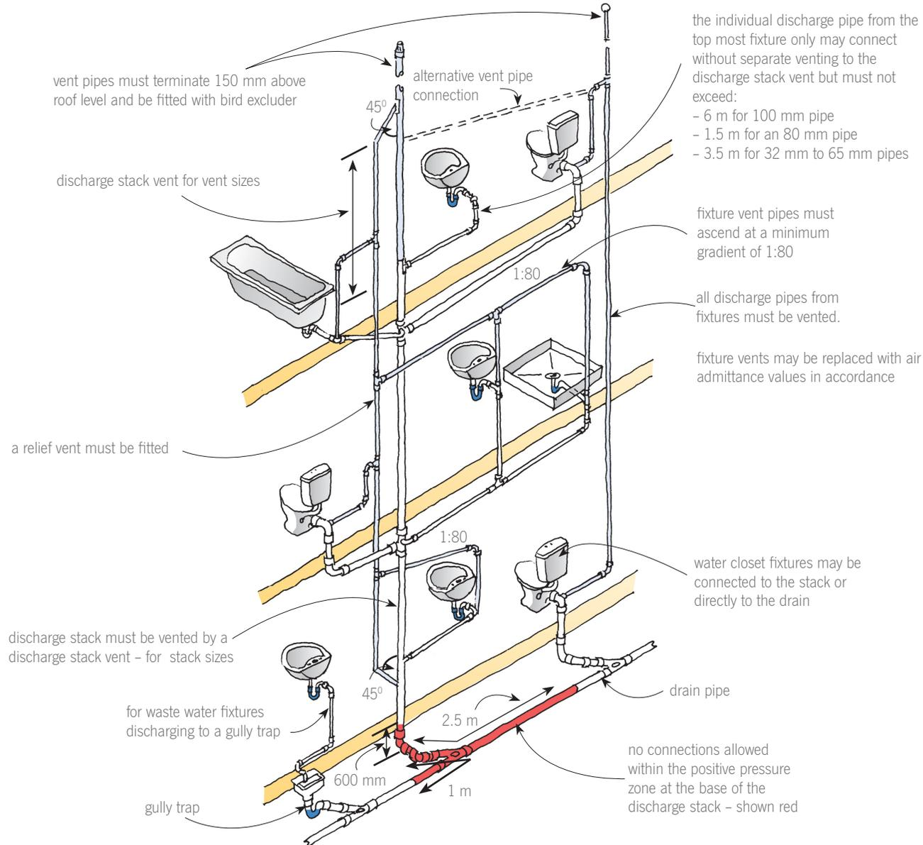
**Basic rules for a system serving three floor levels**
