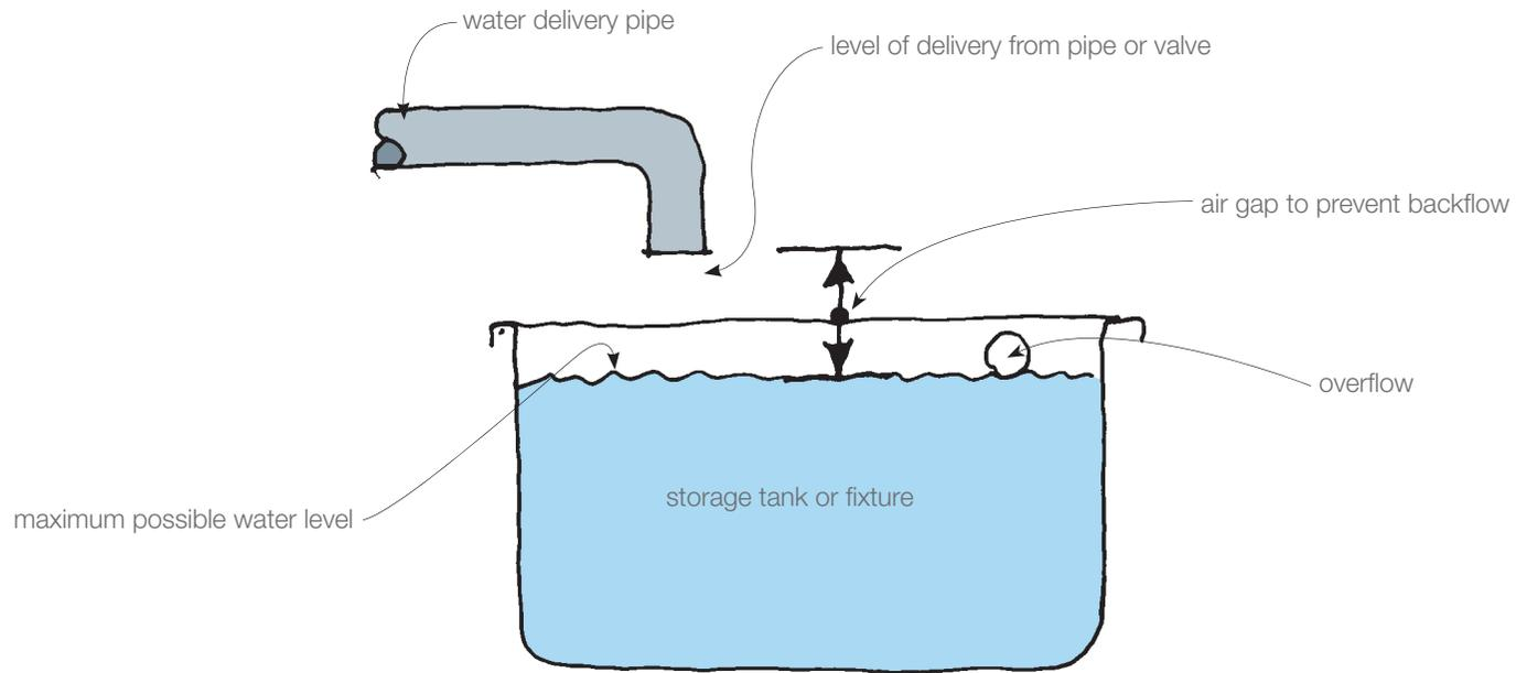
**Principle of air gap used for backflow prevention**
