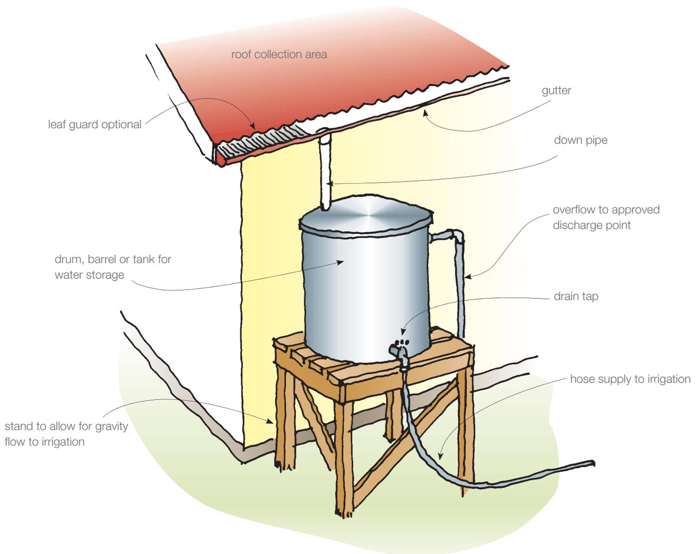
**Simple rainwater storage tank for garden irrigation**
