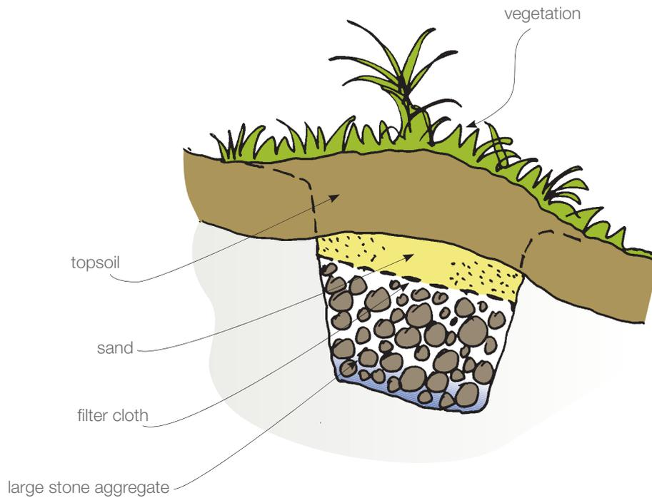
**Subsoil gravity-fed irrigation trench**
