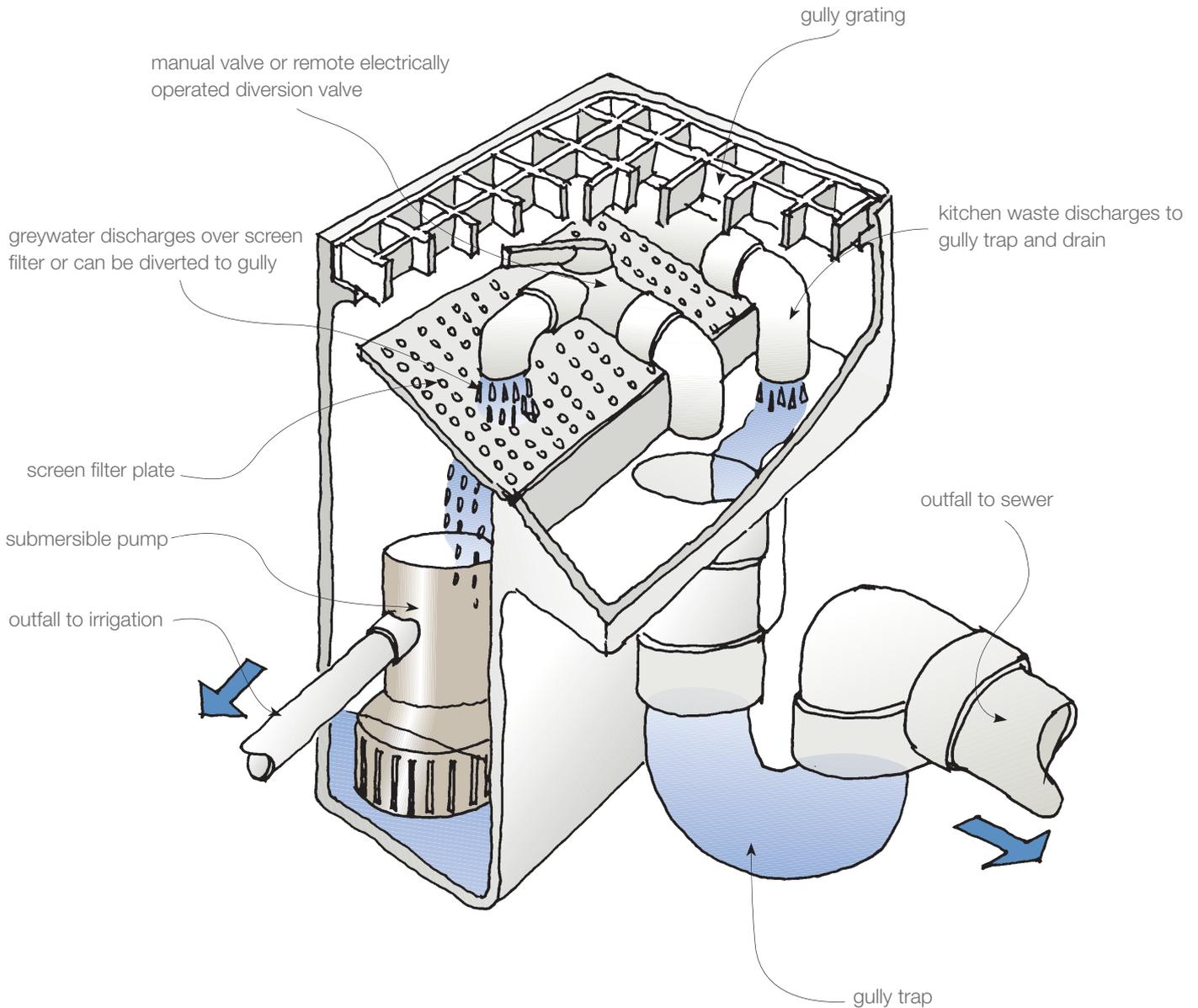
**Cut away schematic diagram of manufactured gully with pumped diversion to irrigation**
