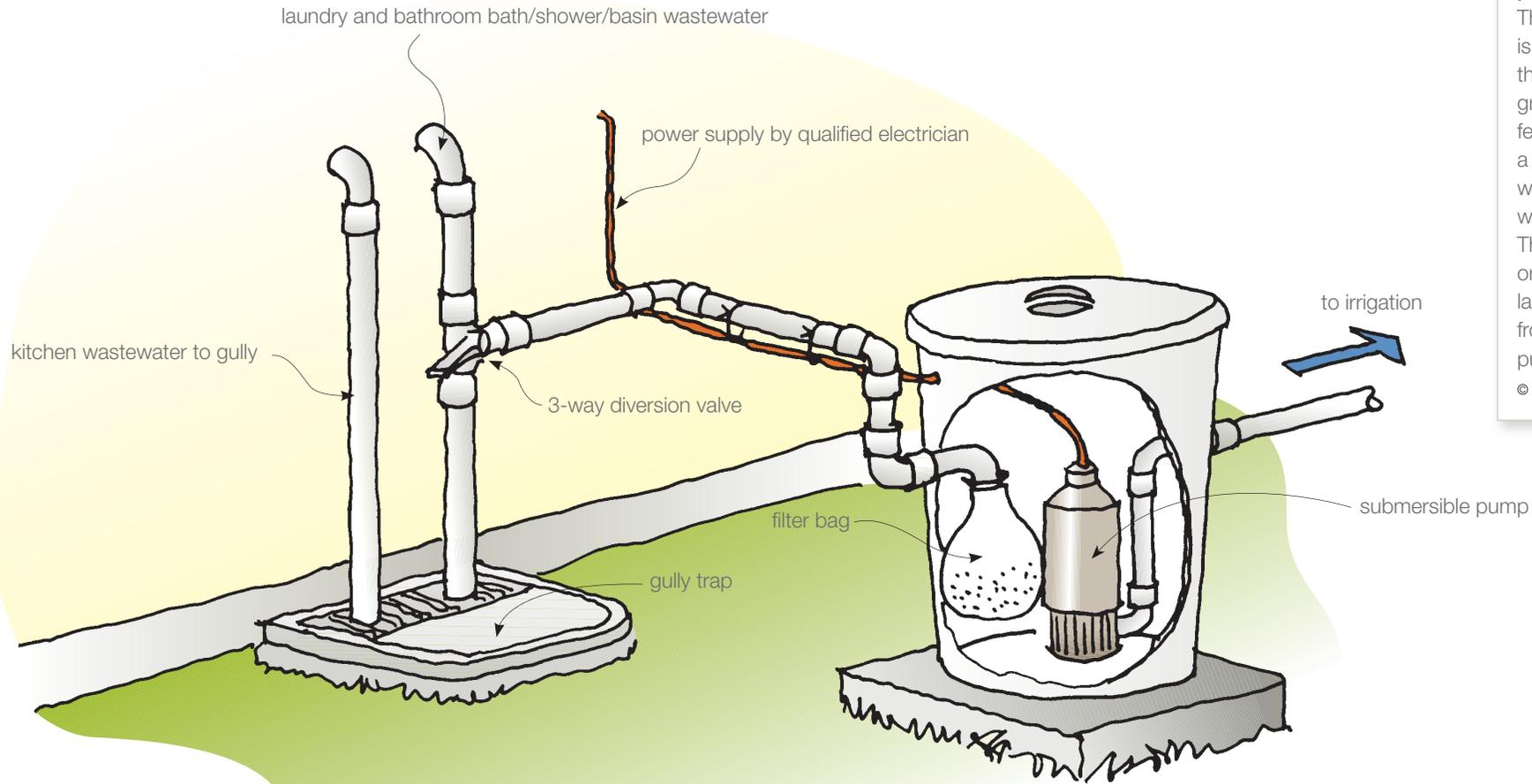
**Diversion of laundry and bathroom greywater for pumped irrigation**
