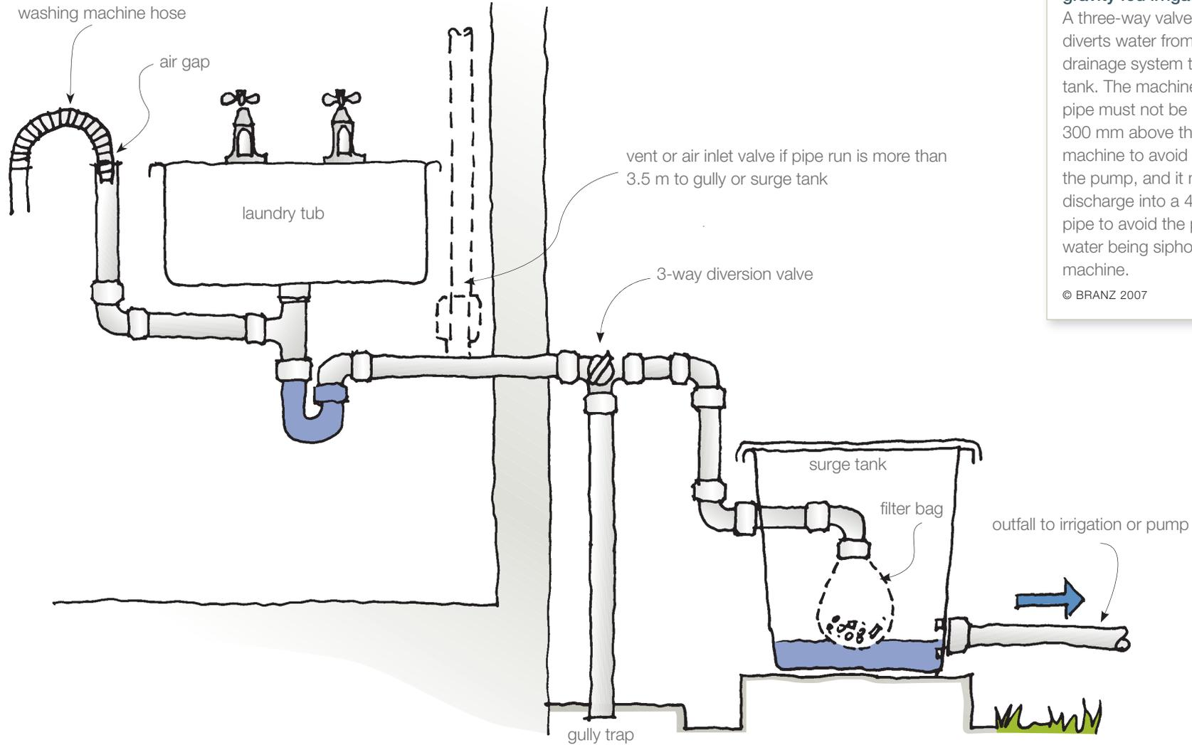
**Diversion of water from washing machine or tub for gravity fed irrigation**
