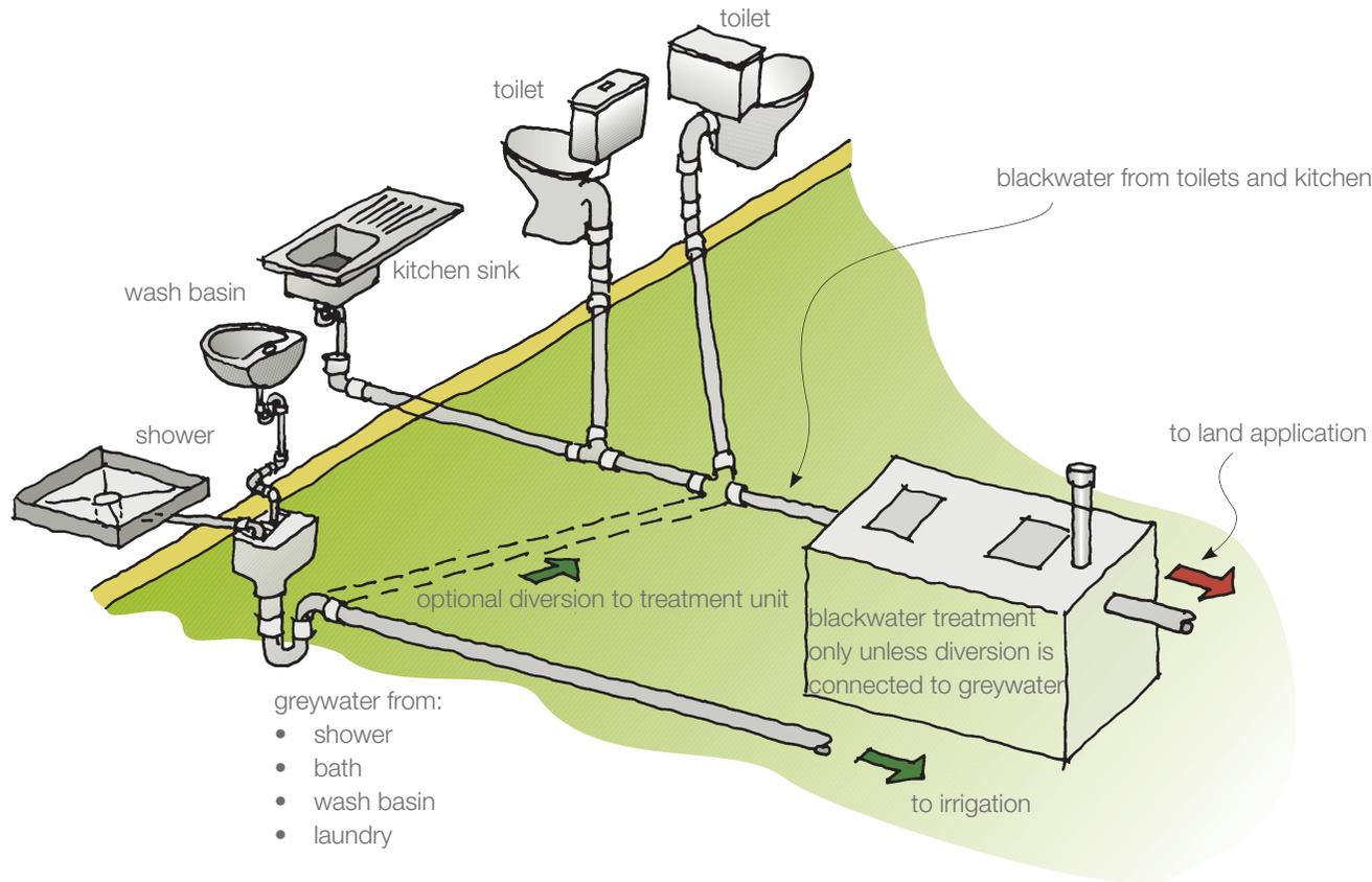
**Schematic of separate on-site domestic greywater and blackwater treatment systems**
