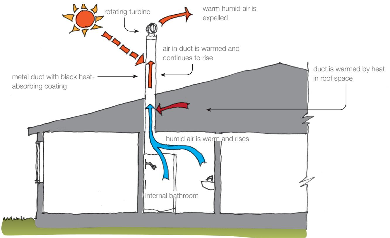
Principle of a solar chimney.
