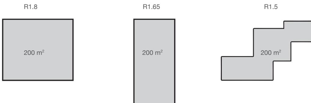
Effect of concrete slab shape on R-value.
