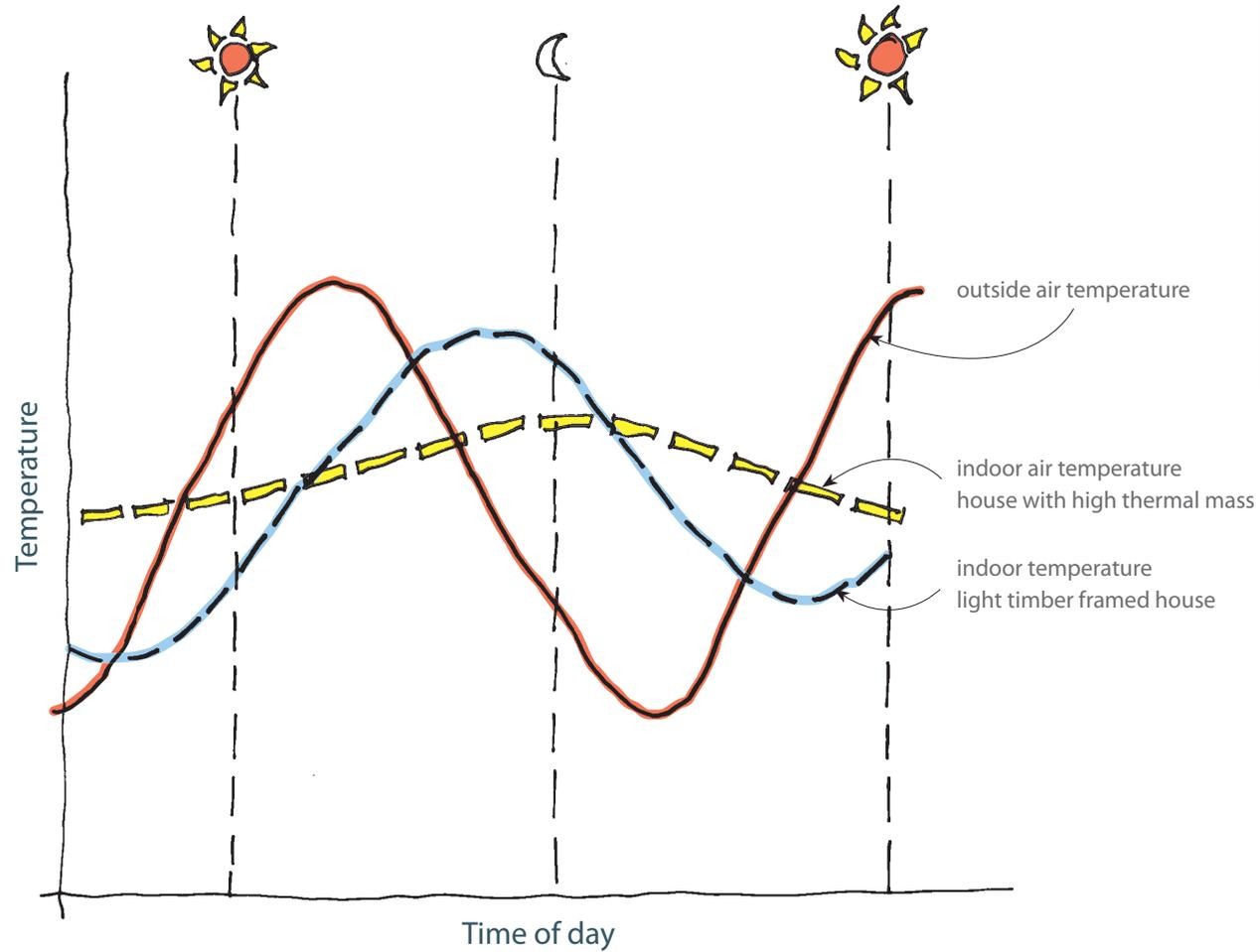
How thermal mass evens out temperature fluctuations
