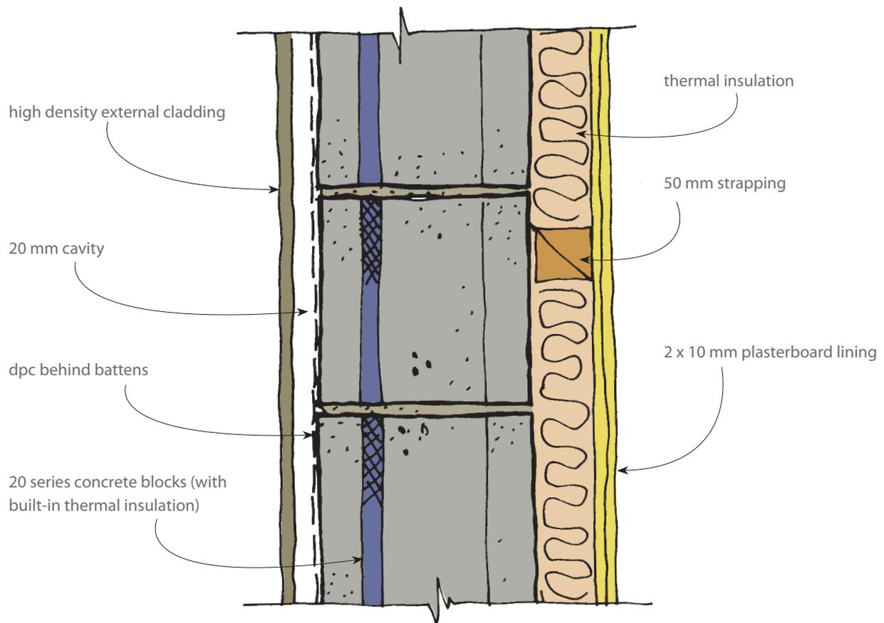
**External sound envelope (concrete masonry)**
