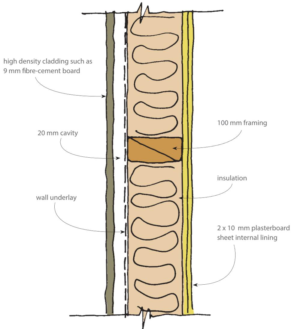
**External sound envelope (fibre-cement cladding)**
