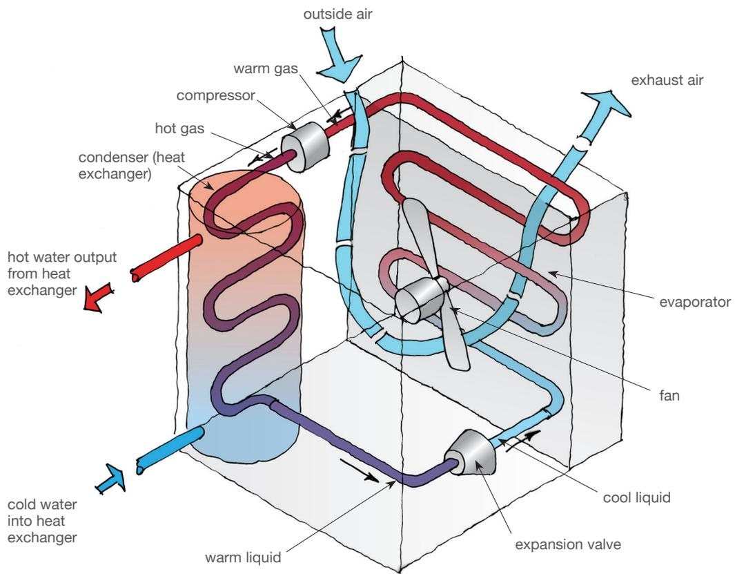
Heat pump water heater cycle.
