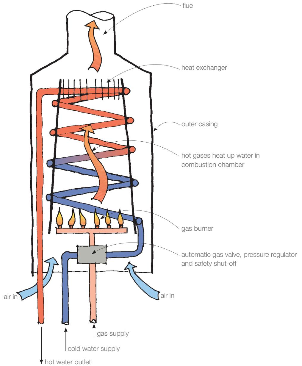
Operation of typical gas continuous flow water heater
