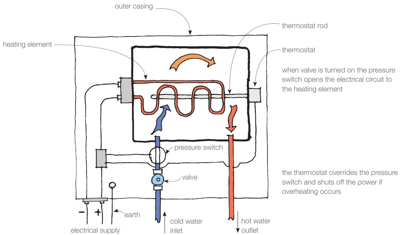
**Operation of typical electric instantaneous water heater**
