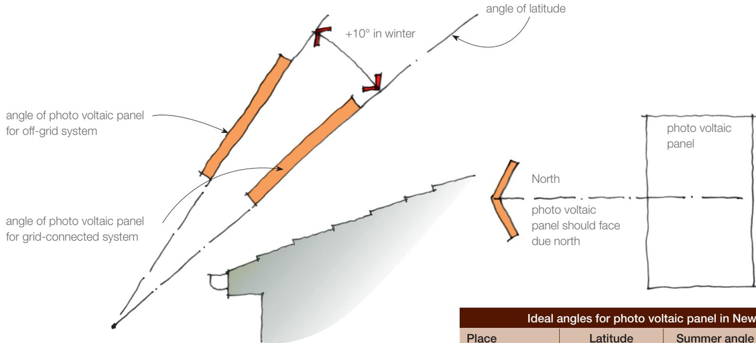
**Photo voltaic panel tilt angle**
