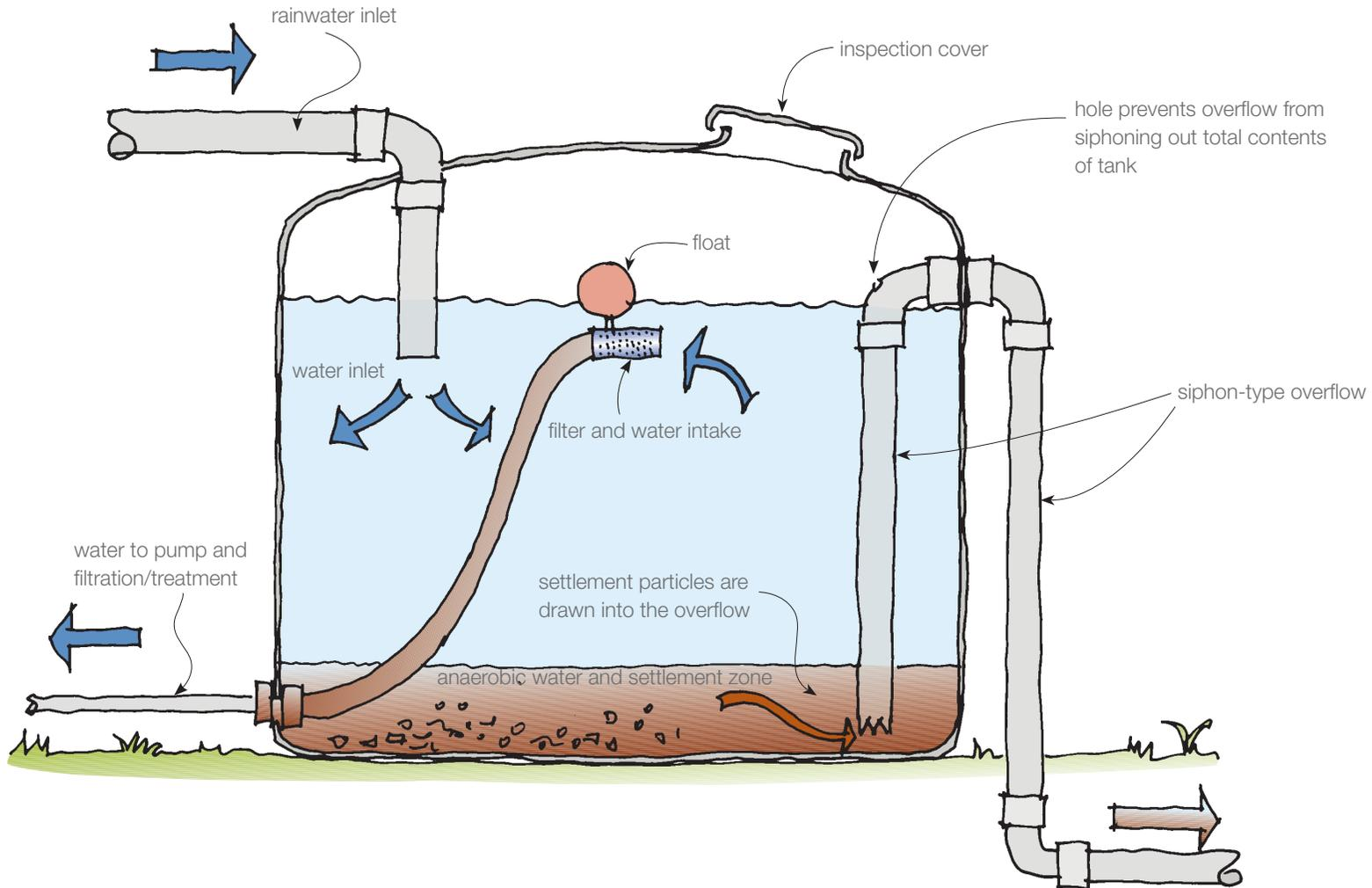
**Schematic drawing of storage tank features that help to deliver clean water**
