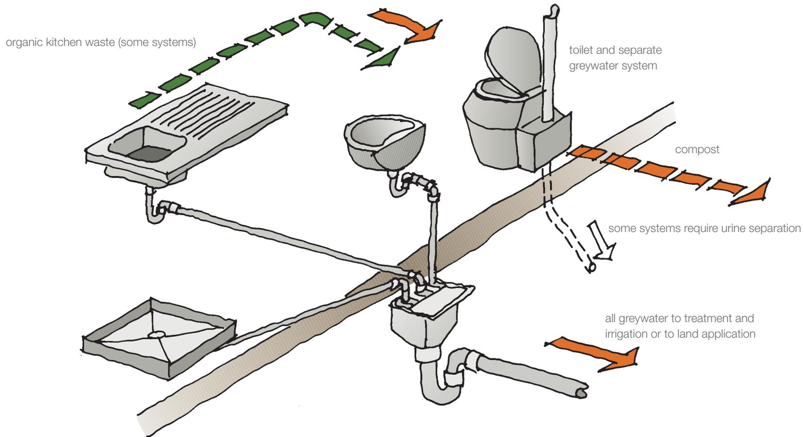
**Schematic of an on-site domestic greywater treatment system used in combination with a waterless composting toilet**
