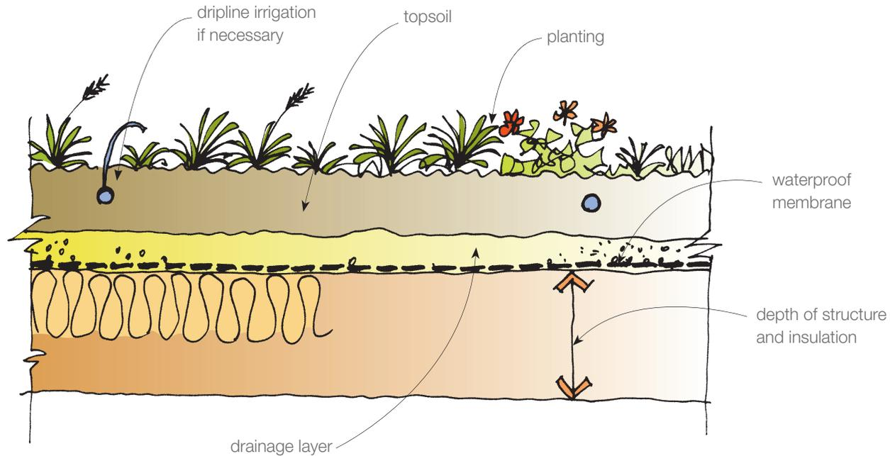
**Cross section of a green roof**
