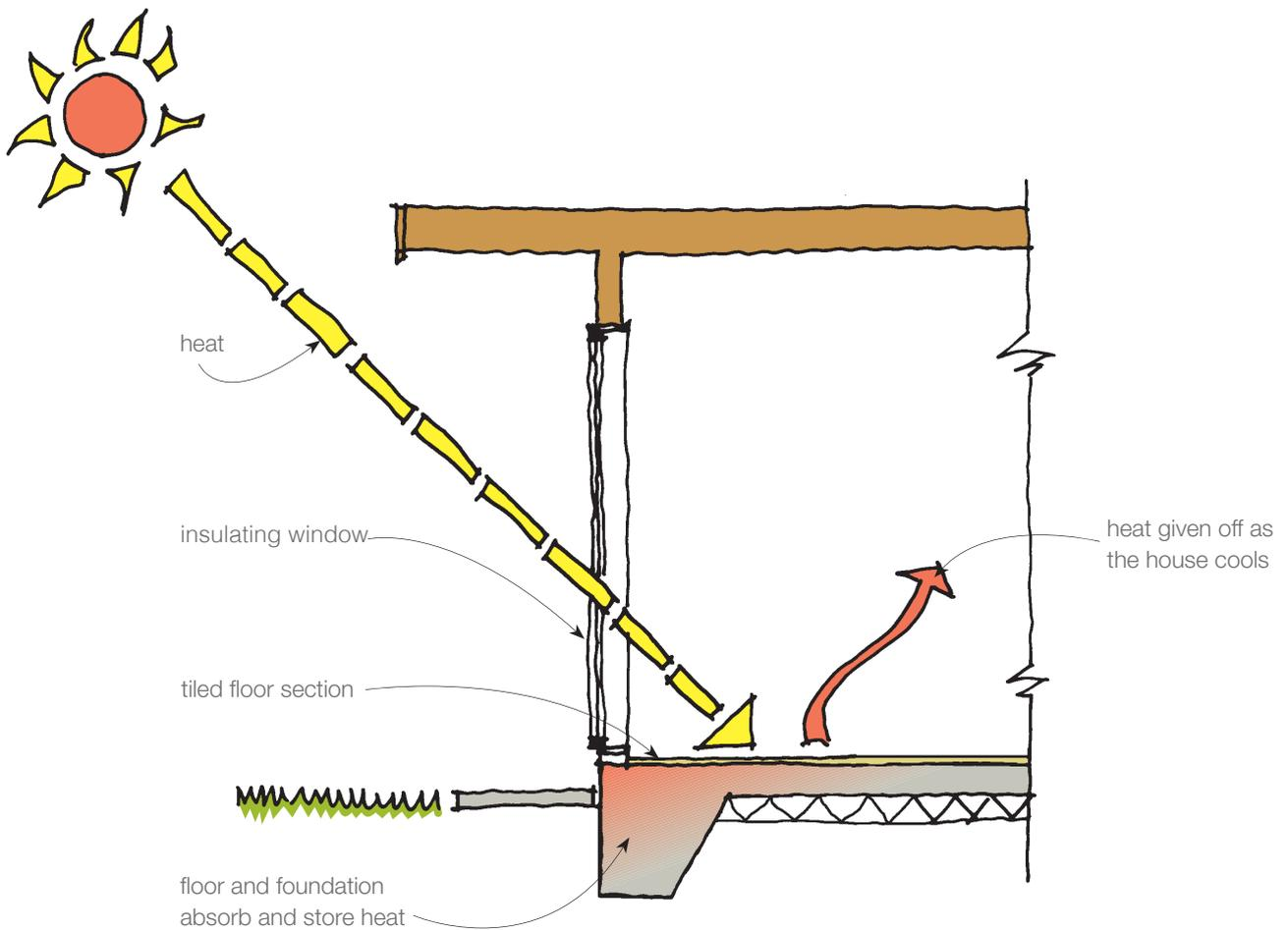
**Principle of using the thermal mass of a concrete floor**
